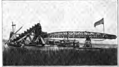
Fig. 6.—Light-draught dredger, with delivery apparatus working round an arc of 210^{\circ} , by Hunter & English.
