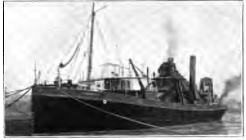
Fig. 4.—Stern-well hopper-dredger "La Puissante," by Wm. Simons & Co. Length 275 ft., breadth 47 ft., depth 19 ft.
