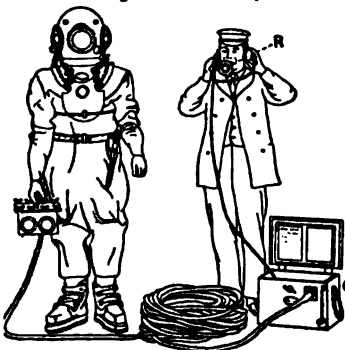
FIG. 4.—Diver's Telephone Communication with the Surface. Q, Battery, with switch and bell in case. R, Attendant's receiver and transmitter.
