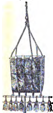
FIG. 15.—Deep-sea Dredge, with Tangle Bar.
